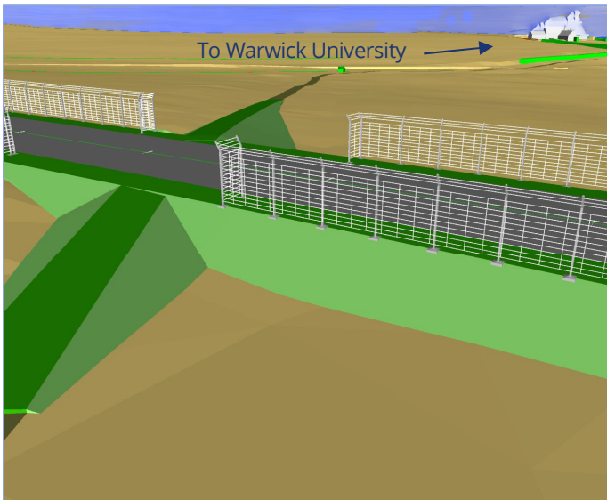
3D visualisation showing fenced off haul route and managed crossing of the Connect 2 cycle path between Kenilworth and Warwick University.
